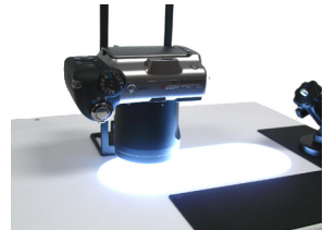
Camera positioned straight down, looking into the inside of the lighting system with fluorescent lights on
