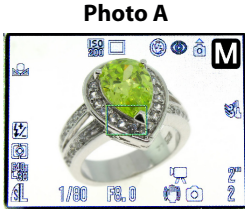
Photo A Focusing at the center of the item (No depth of field achieved) Bottom of ring is not focused
